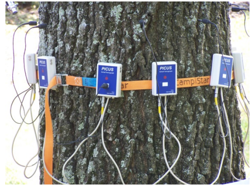
Figure 19. PiCUS tomography listens to the movement of sound through the tree and draws a picture of the tree's internal structure.
