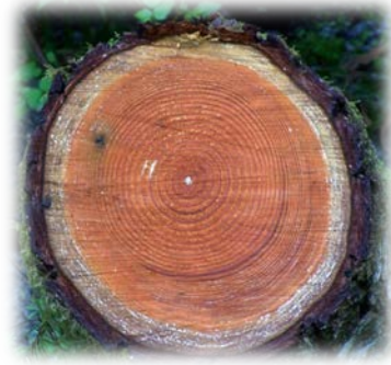
Figure 1. Cross section of a Douglas-fir. The light colored outer ring of wood is the sapwood. The dark wood in the center is the heartwood.
